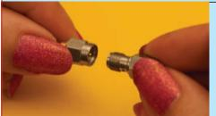
1. Convert your standard cable assembly into a Push-On Assembly by threading the standard female side of the adapter onto the male connector of the assembly.
