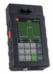
▲ Fig. 1 E-Band spectrum analyzer.
