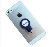
▲ Fig. 2 Near field adapter connected to a smartphone.
