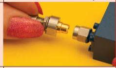
4. To disconnect, just pull the connector off.
