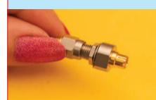
2. Your standard SMA male cable assembly is converted to a Push-On SMA female Cable Assembly.
