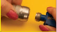
6. Keep fingers on "Back Nut" to ensure that "Lock Nut" cannot slide back and pull the connector off.
